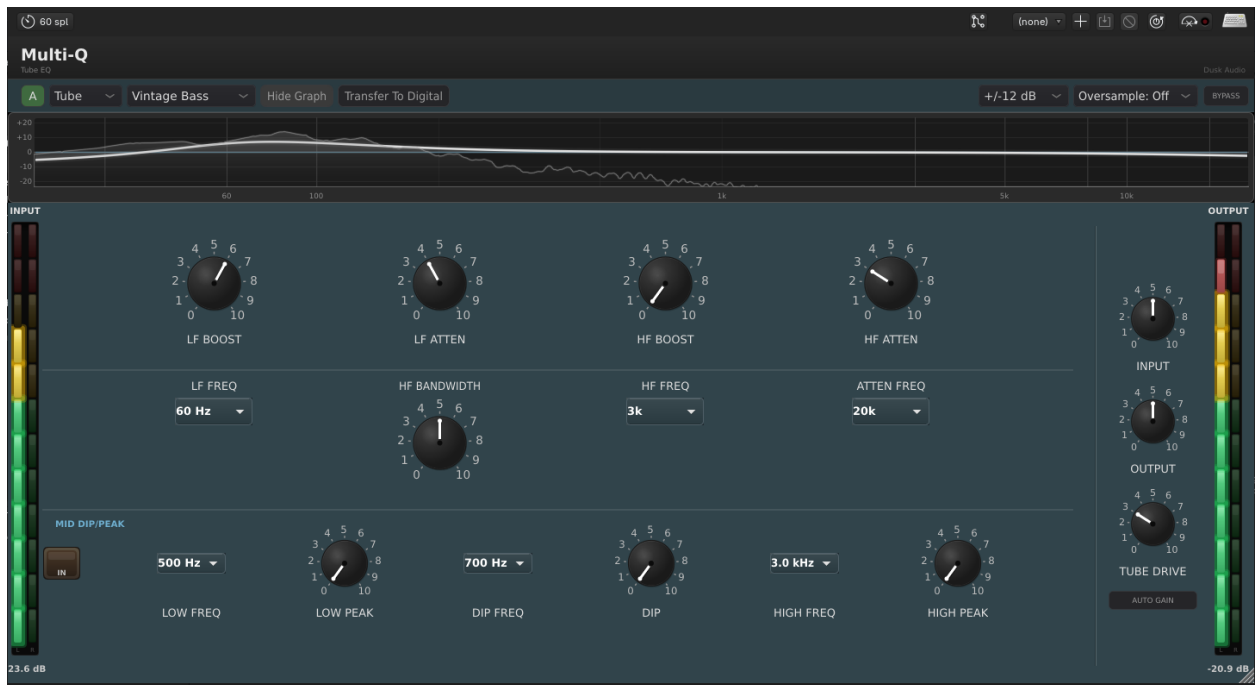
Figure 9: Multi-Q in Tube mode with boost+cut at 60 Hz
