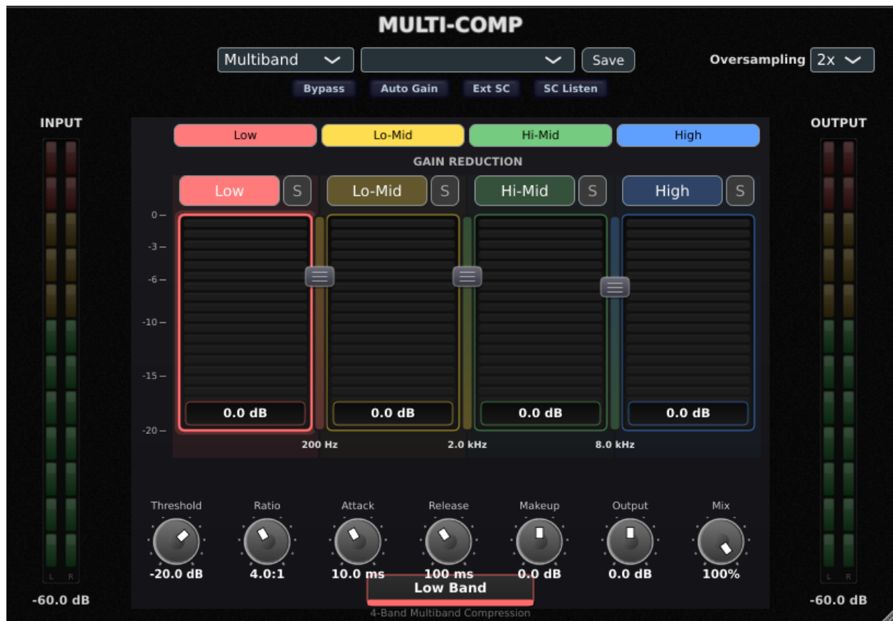
Figure 3: Multiband mode default 4-band layout
