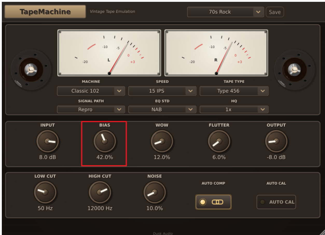
Figure 15: Bias control with Auto Calibration off
