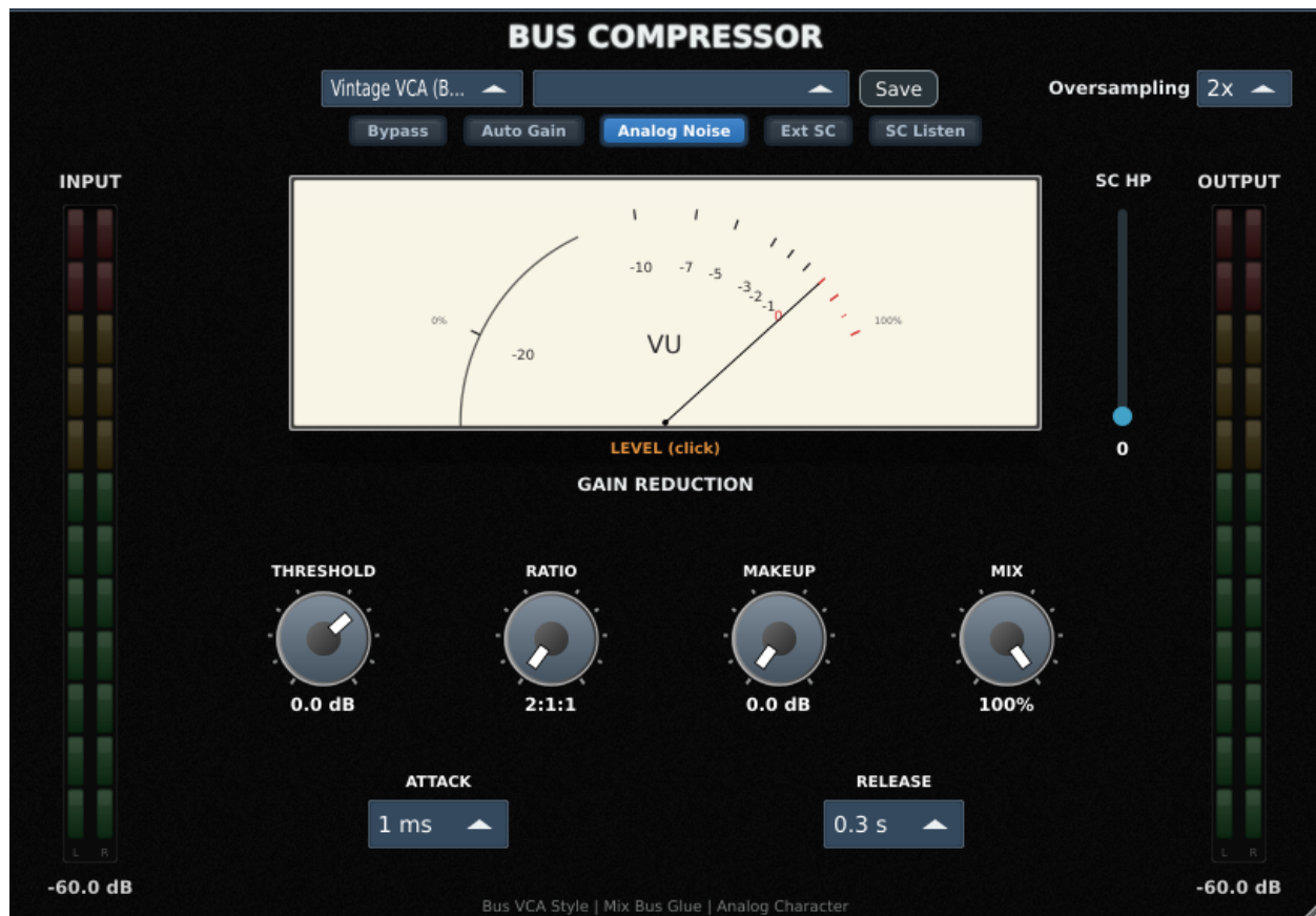
Figure 2: Bus Compressor with Classic Drum Glue settings
